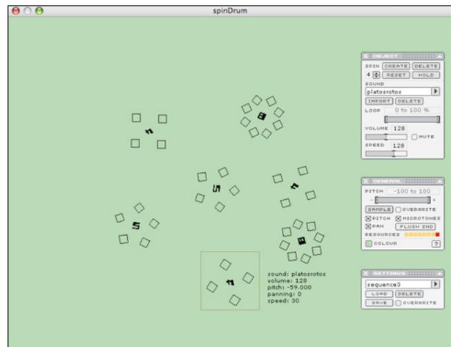
**Figure 2: SpinDrum.** Each wheel contains from 1 to 10 pedals. The wheels rotate in various speeds, and when a pedal hits top position (12 o'clock) it triggers the sample or sends out OSC info to the soundengine. This allows for the creation of complex polyrhythms. The X and Y location of the wheels can affect parameters such as pitch and panning.
